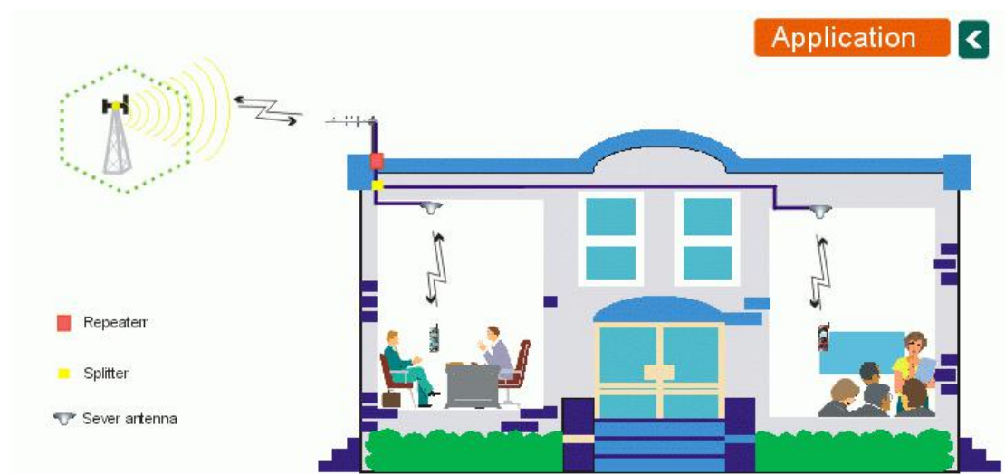
Figure 2.1 Wireless repeater application diagram
