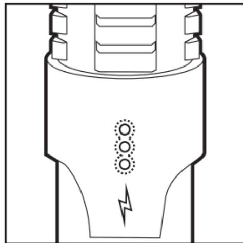
To set the laser to **full-power/momentary mode**, hold the SmartSwitch and press the tailcap button. After unlocking the laser, the 3 LEDs will be lit up.
