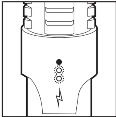
To switch to **medium-power mode**, you may hold the SmartSwitch button until the 2nd LED lights up.
