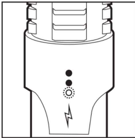
To unlock the laser you only need to **push the SmartSwitch quickly three times and then hold it for less than 1 sec. two times.**
