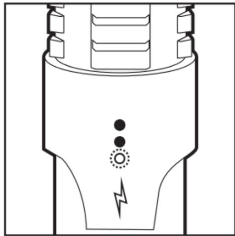
After pressing the power-button on the tail cap, the laser is now waiting for the unlocking code to be entered. 1 LED light will be blinking to indicate this.
