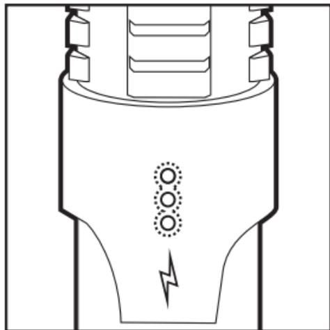
To switch to **high-power mode**, you may hold the SmartSwitch button until the 3rd LED lights up.
