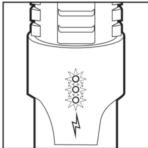
From any mode, 1 quick click will put the laser into **tactical standby mode**. The 3 LED lights will start flashing to show the laser is on stand-by.
