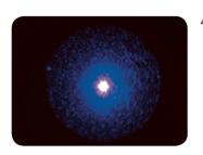
**Moisture** - We do not recommend using any laser products in highly humid or foggy conditions. If your laser unit is used in these conditions and/or submerged in water, the beam may appear similar to the above picture. You will not be able to clean this as water has condensed inside the lens and/or crystal set. This condition can be repaired by Wicked Lasers, however, will not be covered in your warranty. A repair cost will apply.
