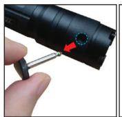
Removing the Safety Interlock from the Endcap will disable the laser.
