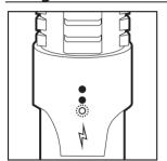
After pressing the power-button on the tail cap, the laser is now waiting for the unlocking code to be entered. 1 LED light will be blinking to indicate this.
