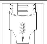
From any mode, 1 quick click will put the laser into **tactical standby mode**. The 3 LED lights will start flashing to show the laser is on stand-by.
